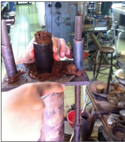
Gambar 2.1 Proses pencetakan sampel uji undisturbed
